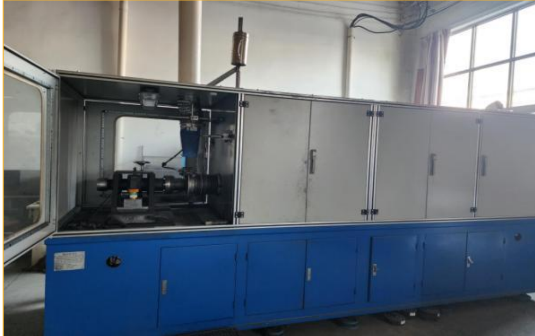
Brake pad inertia bench test machine
